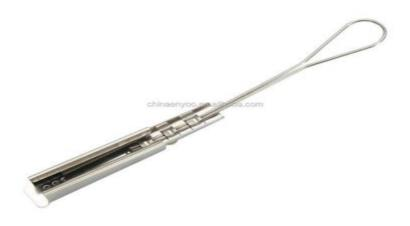
Optical Drop wire Anchoring Connecting Clamps Consist of three basic parts body, wedge and shim. hard aluminium body, shim and wedge, with a stainless-steel wire bail. The Drop Wire Clamps secures dead-end telephone drop wire at pole or building and provides long corrosion-free service.
