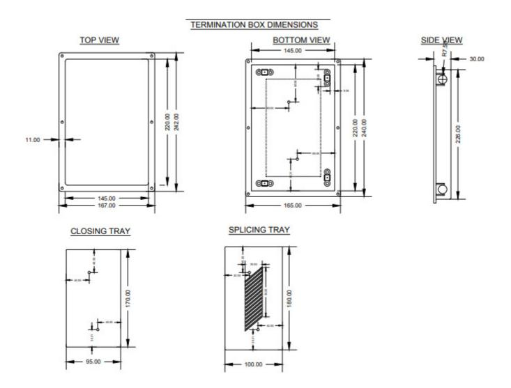
Fiber termination box (FTB) generally refers to the box shape fiber optic management products used to protect and distribute the optical fiber links in FTTH Networks. The direct application of termination box is to terminate fiber optic cables and connect the core of the cable and patch cord. The Fiber termination box as following
