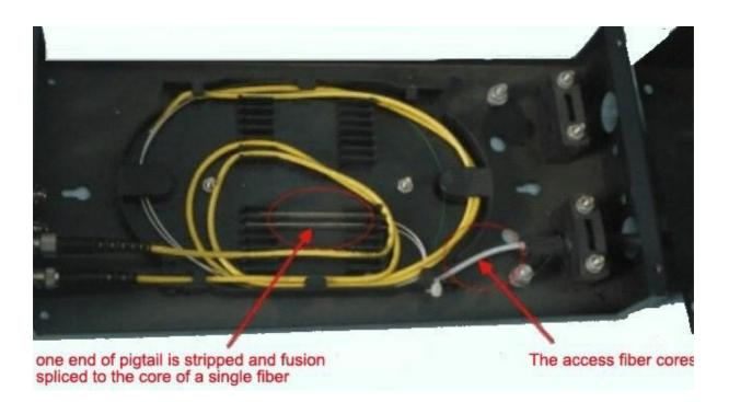
As the picture shows, the access fiber cables can be multi-core. For example, a 4- fibers fiber optic cable (namely fiber optic cables with 4 cores), then, after this fiber optic cable accessing to the termination box, it can be splice into for 4 fiber patch cords. The picture above shows 2 pigtails, so that they lead to 2 fiber patch cords.
