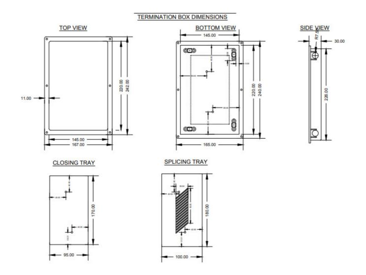
Fiber termination box (FTB) generally refers to the box shape fiber optic management products used to protect and distribute the optical fiber links in FTTH Networks. The direct application of termination box is to terminate fiber optic cables and connect the core of the cable and patch cord. The Fiber termination box as following
